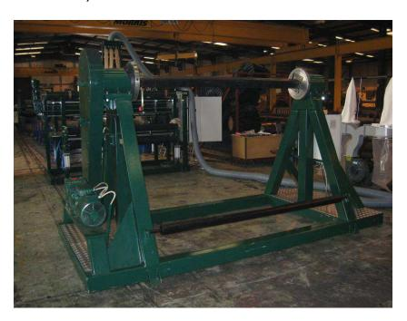
The ITBBM can be supplied with a belt re-winder which can be running synchronic with the Belt Buffing Machine. This is realized by an optical eye, measuring the distance of the belt, and keeps on re-winding as the ITBBM is transporting the belt through the machine.
