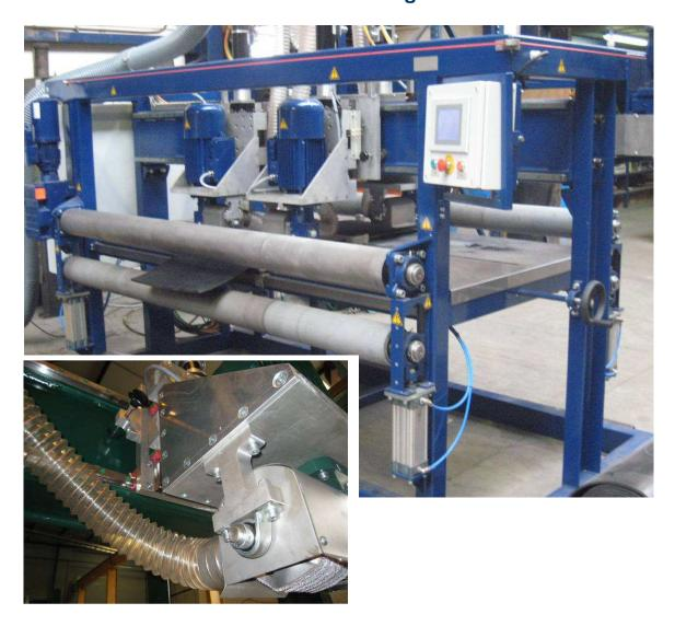
The ICE-Trade Belt Buffing Machine (ITBBM) is developed to grind (buff) the conveyor belt, there where cleats and or sidewalls must be installed. The ITBBM features 3 grinding heads: 2 for length wise buffing for the sidewalls, I buffing head, crosswise, for the cleats.
