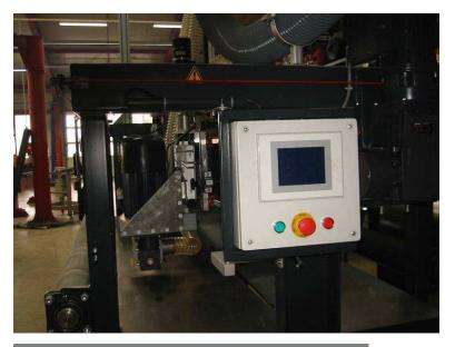
The ITBBM is operated with a touch screen, where all the settings can be made.
