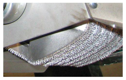
The grinding wheels, installed to achieve the optimum buffed surface for good bonding properties are 6 Vane Wheels, with SSG ® grit Tungsten carbide.
